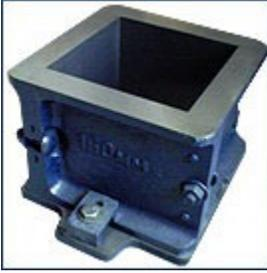
For cube test two types of specimens either cubes of 15cm X 15cm X 15cm or 10cm X 10cm x 10cm depending upon the size of aggregate are used. For most of the works cubical molds of size 15cm x 15cm x 15cm are commonly used.
